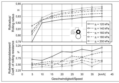
Fig.2: Coefficients of rolling resistance (at ~ 1% slip) as well rolling radii of a standard tyre Goodyear 18.4 R 38 on the roller test rig as a function of tyre pressure and speed. Static axle load: 24.6 kN
