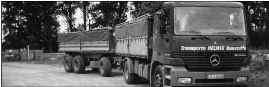
Fig. 2: train with two-axle truck and a three-axle trailer, each tipping construction
