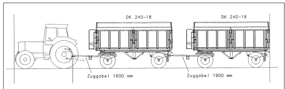
Fig. 1: train with tractor and two trailers, each with 18 t max. permissible weight
