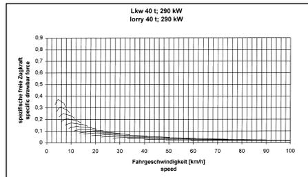
Fig. 3: Specific tractive power driving speed diagrams for tractor train (left) and for truck train (right)
