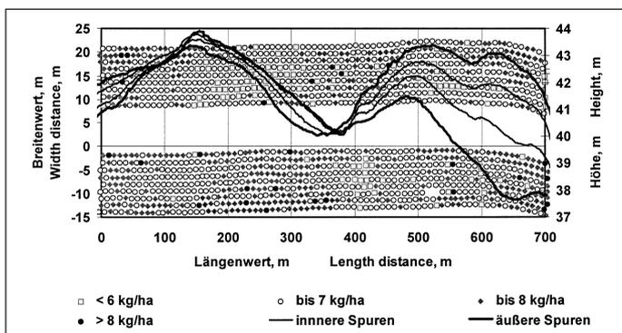
Fig. 3: Area specific fuel consumption for ploughing on the site 803 and the height profile of the innermost and outermost passages
