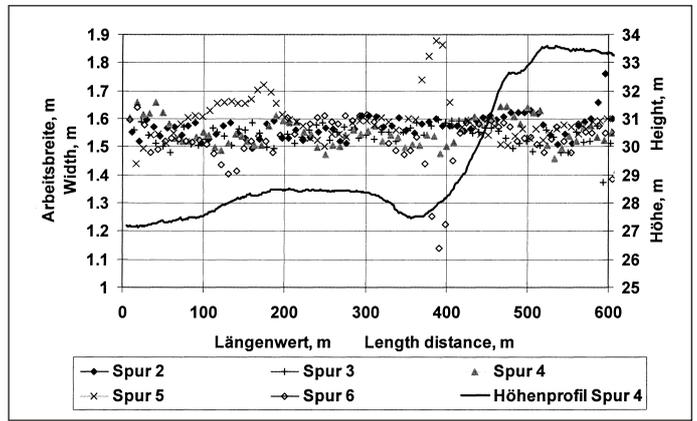
Fig. 2: Working width at ploughing (tractor drives in the furrow) for adjacent passages on the site 804
