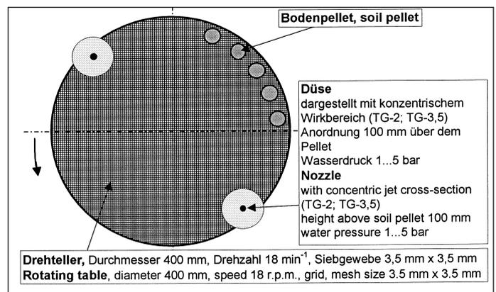
Fig. 1: Test equipment for dissolving soil pellets by spraying nozzles
