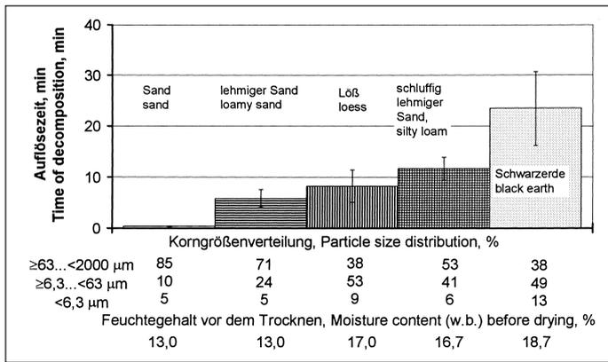
Fig. 2: Dissolving time of dried soil pellets in silent water ( $t = 15\text{ }^{\circ}\text{C}$ )
