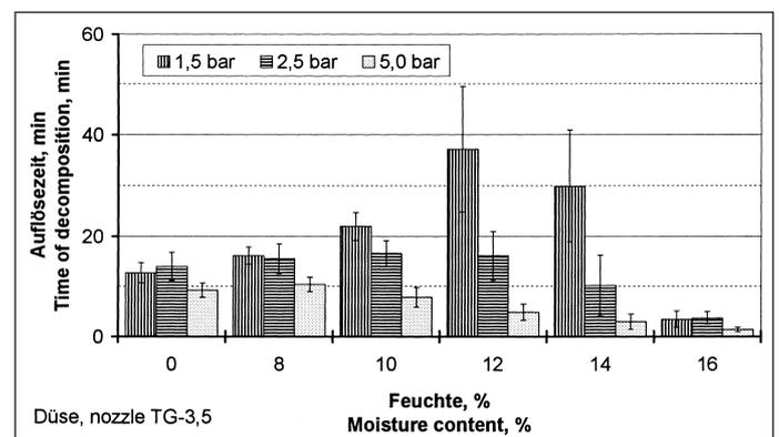
Fig. 4: Dissolving time of soil pellets under a water jet depending on moisture content and water pressure (nozzle TG-3,5)
