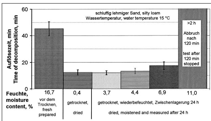
Fig. 3: Dissolving time of silty-loam sand pellets in silent water depending on moisture content
