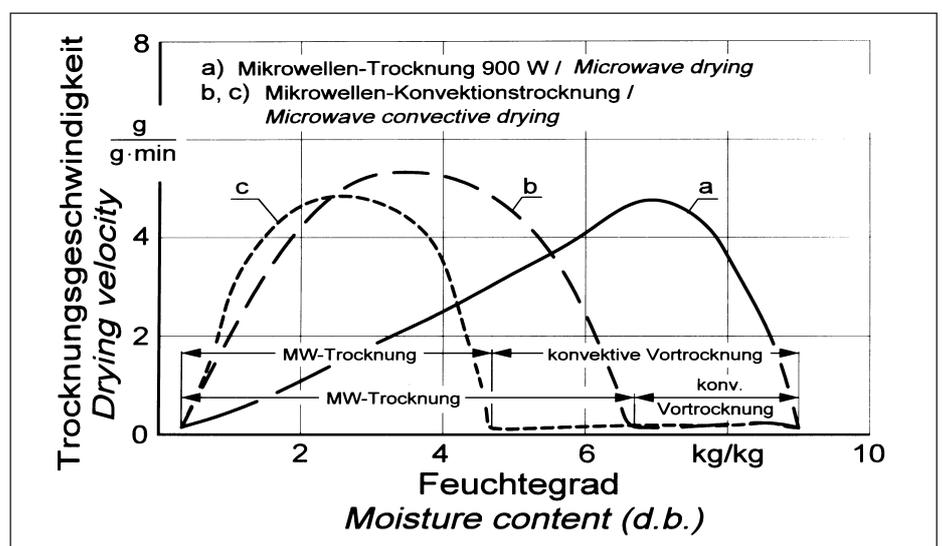
Fig. 1: Drying behaviour of carrot slices (1.5 mm) by microwave drying and microwave drying with convective pre-drying
