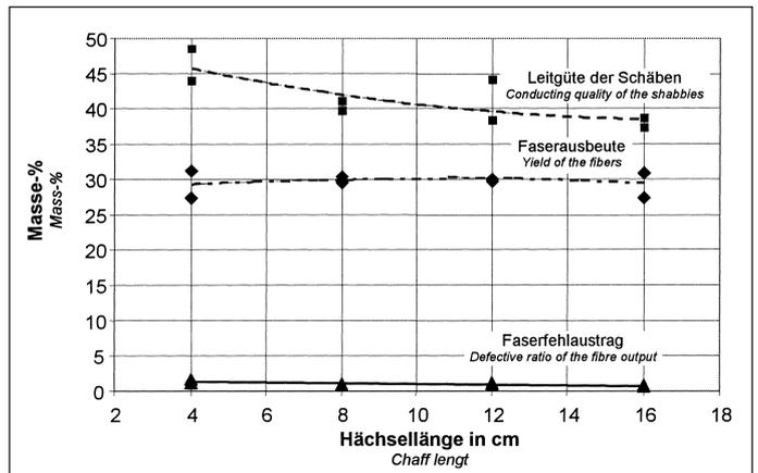
Fig. 2: Fiber yield, defective ratio of the fibre output and conducting quality of the shives vs. chopped length (Free area of the sieves: 0.23; lid inserts: roof conducting facility and fidding flat; circumferential velocity of the hammers: 49 m/s, mass flow: 1 t/h)
