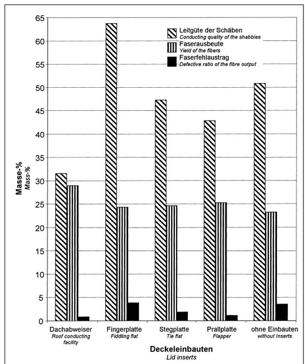
Fig. 3: Fiber yield, defective ratio of the fibre output and conducting quality of the shives vs. lid inserts (Free area of the sieves: 0.23; chopped length: 8 cm, circumferential velocity of the
