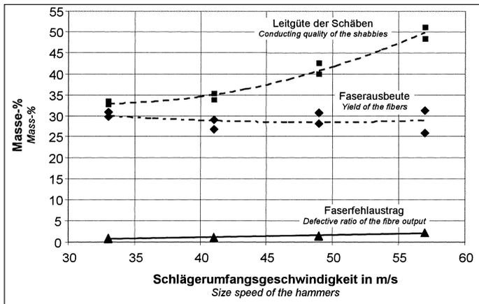
Fig. 1: Fiber yield, defective ratio of fibre output and conducting quality of shives vs. circumferential velocity of the hammers (Free area of the sieves: 0.23; lid inserts: roof conducting facility and fidding flat; chopped length: 8 cm, mass flow: 1 t/h)
