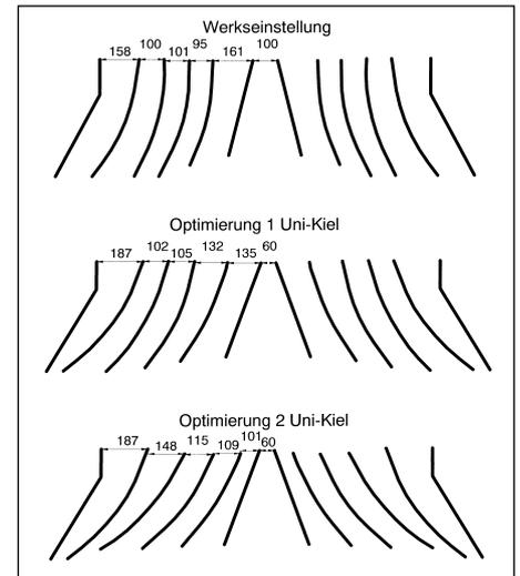
Fig. 5: Entrance slits (mm) between guiding plates of the chopper with 6.3 m working width
