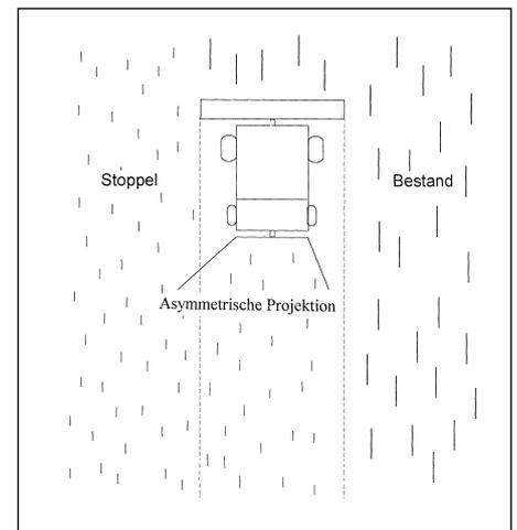
Fig. 6: Unsymmetrical projection by the guiding plates
