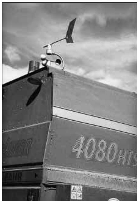
Fig. 8: Sensor for recording wind direction and wind speed
