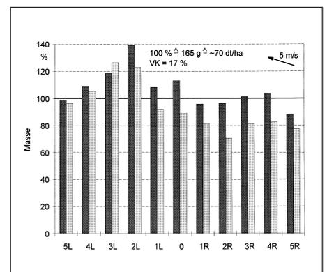
Fig. 2: Good lateral distribution at 6.1 m working width (11 recording points, 0 in the middle of combine, 2 repetitions)
