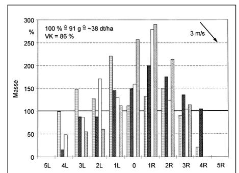
Fig. 3: Insufficient lateral distribution at 6.1 m working width (11 recording points, 0 in the middle of combine, 4 repetitions)
