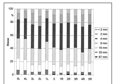
Fig. 7: Sieve fraction of test run (circular openings: 2 - 67 mm)
