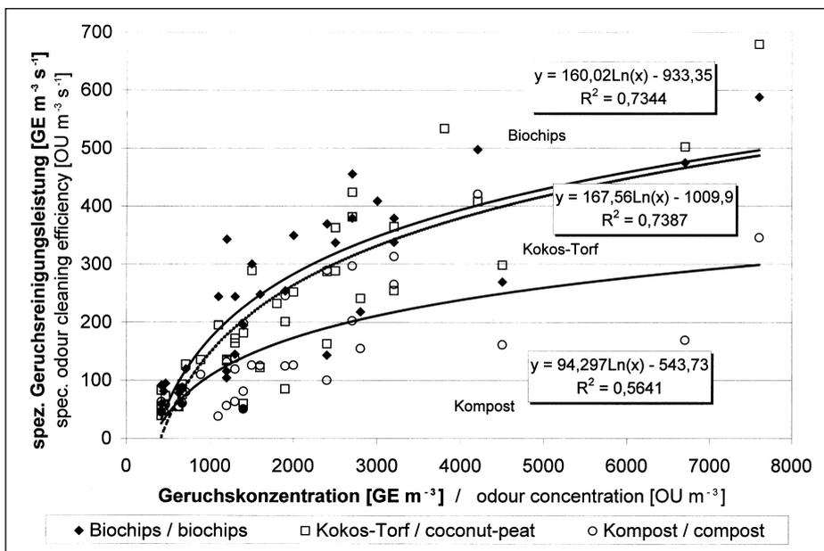
Fig. 1: Relation between the specific odour cleaning efficiency and the odour concentration in the waste air
