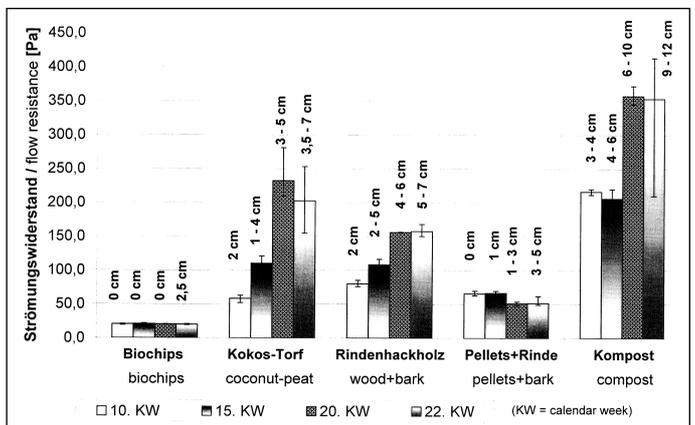
The specific filtering performance [ $\text{W}/1000 \text{ m}^3$  of expedited air] in the last three weeks of the trial was around 30% less for Biochips compared with the coconut fibre peat. This applied only for the radial fans used in the trial. For all the other biofilter plants, the filter performance has to be calculated anew from their air throughflow and the appropriate flow resistance of the plant as well as the fan performance characteristics.
