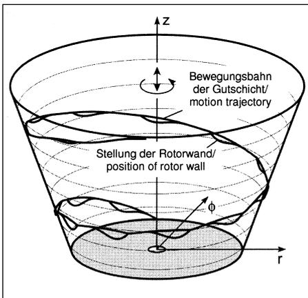
Fig. 2: Computed motion trajectory of rotary cleaning system
