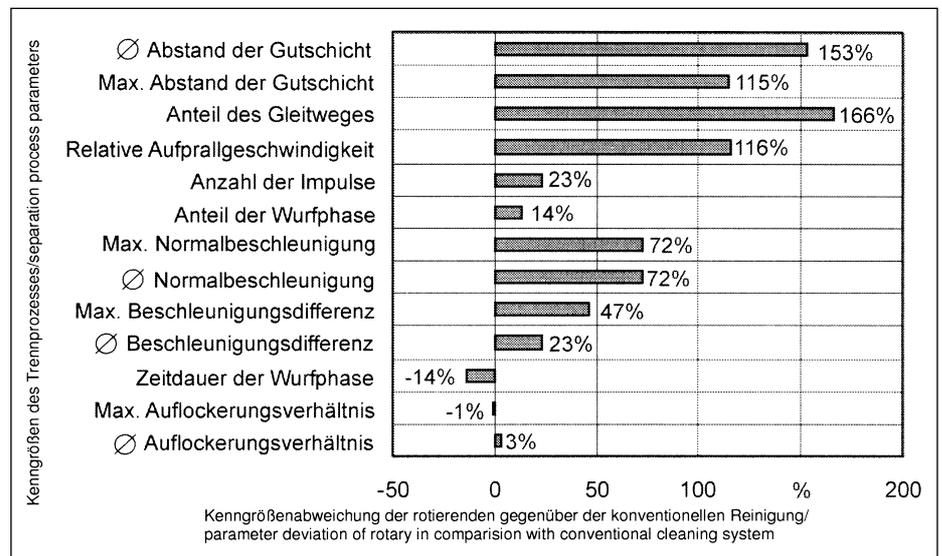
Fig. 4: Parameter deviation of rotary in comparison with conventional cleaning system
