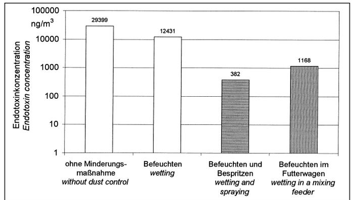
Fig. 3: Airborne endotoxins during littering without and with dust reduction measures
