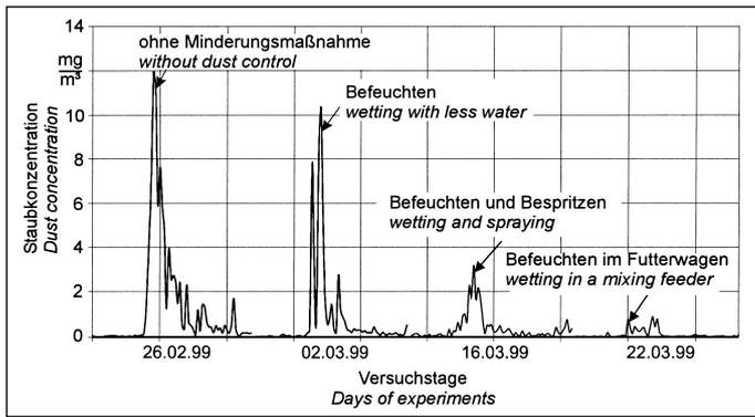
Fig. 2: Course of total dust concentration during littering without a dust reduction measure and various measures for dust reduction
