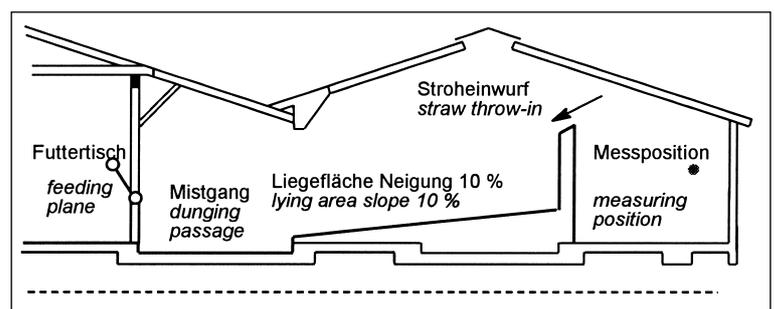
Fig. 1: Scheme of sloped floor housing
