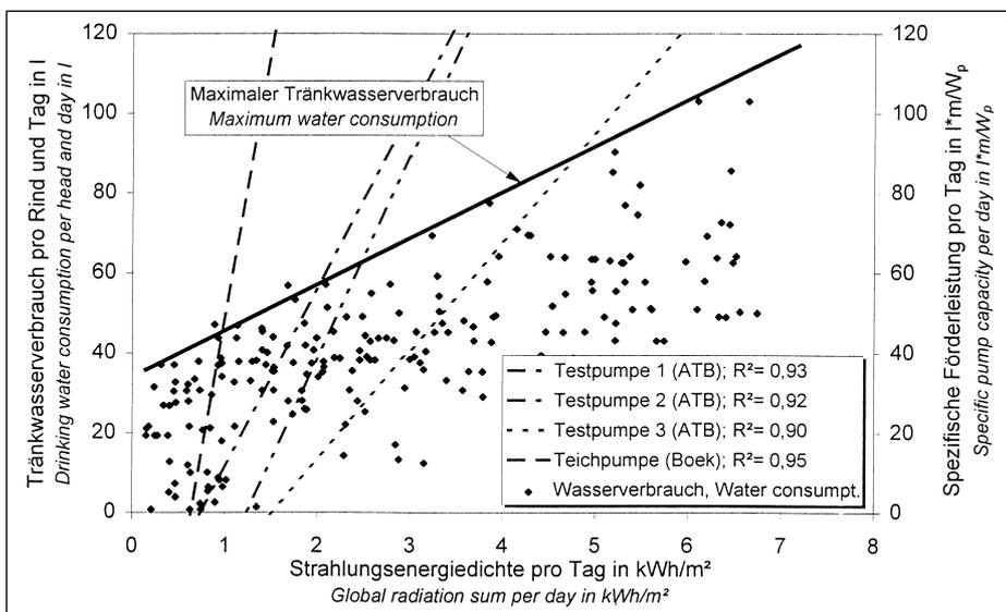
Fig. 2: Drinking water consumption of non-lactating cows and specific capacity of pv-pumps versus global solar radiation intensity
