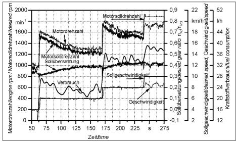
Fig. 2: Reaction of the partial load controller for the three speed sectors whilst ploughing
