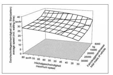
Fig. 1: Average transport<br/>(incl. laid-up time),<br/>depending on maximum<br/>speed determined byonly s<br/>on the<br/>In c<br/>average
