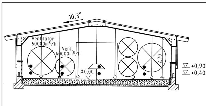
Fig. 2: Measuring cross section, position of heat wire-anemometer •
