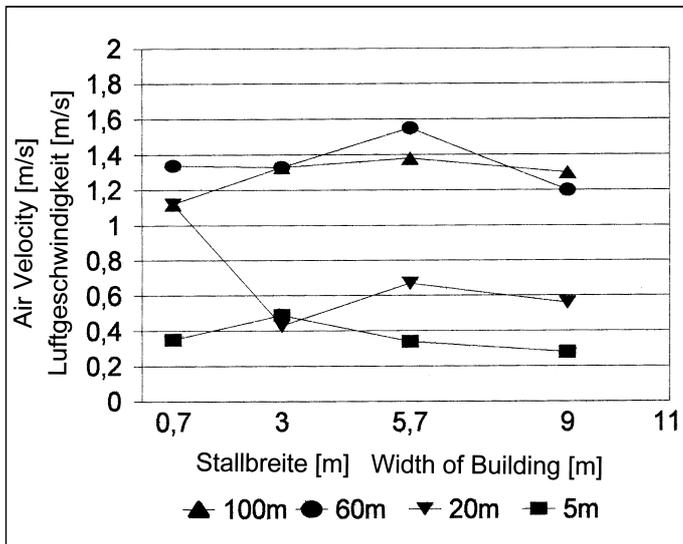
Fig. 3: Air velocity at measuring points of inlet air variant 3
