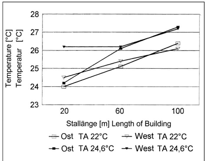
Fig. 4: Distribution of temperatures in axial section
