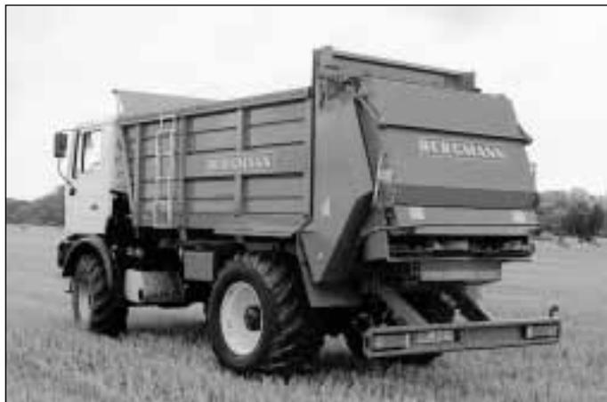
*Spreading unit Bergmann TSW 1616S twin plate broadcast aggregate mounted on a truck with low ground pressure tyres*
