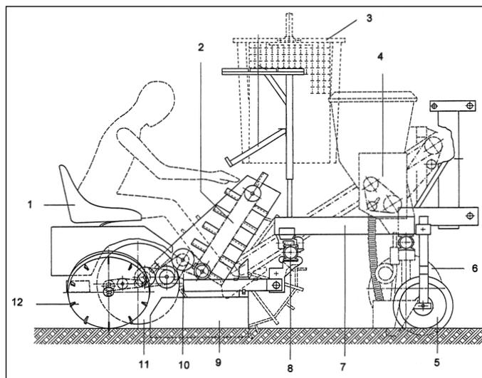
Fig. 1: Planting machine requirements based on a clamp disc machine with chain and cup magazine: 1. ergonomically-designed work position, 2. cup and chain as magazine, 3. storage platform, 4. additional equipment for placed fertilising, 5. steplessly-adjustable front runner wheel, 6. pressure roller for reconsolidation, 7. double frames, 8. plant aggregate extra, 9. plant coulter, 10. synchronised spur gear and chain drive, 11. clamp discs, 12. pressure wheels.
