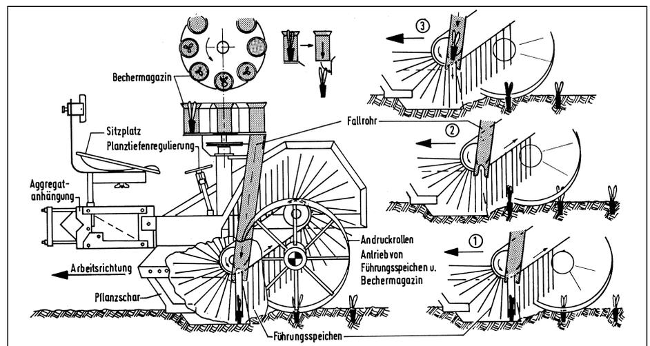
Fig. 3: Planter with revolver-head magazine (plant conveyance directly into the furrow).
