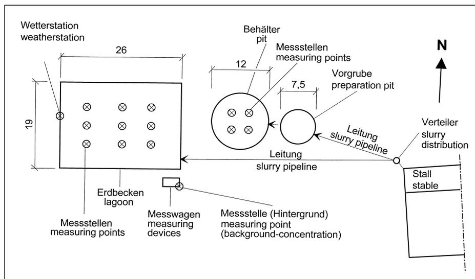
Fig. 1: Slurry pipelines from the stable to lagoon and pit as well as arrangement of measuring points
