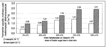
Fig. 3: Fermenter-specific methane yield with rnesophilic and thermophilic fermentation (34 °C) of liquid cattle manure and liquid fodder beet silage under 15 days of hydraulic retention time
