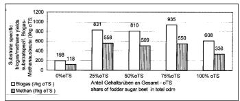
Fig. 2: Substrate-specific biogas/methane yields with mesophilic fermentation (34 °C) with different proportions of liquid fodder beet silage and cattle slurry under 20 days of hydraulic retention time
