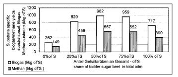
Fig. 1: Substrate specific biogas/methane yields with thermophilic fermentation (54 °C) with different proportions of liquid fodder beet silage and cattle slurry under 20 days of hydraulic retention time
