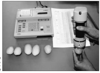
Fig. 2: Determination of potato flesh colour via Minolta ChromaMeter 310
