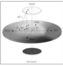
*Fig. 1: Three-dimensional representation of the L\*a\*b\* colour system*
