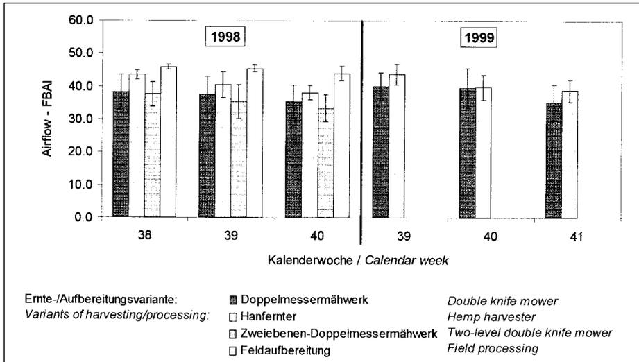
Fig. 2: FBAI-values of processed fibre bundles during field lying period after mowing.
