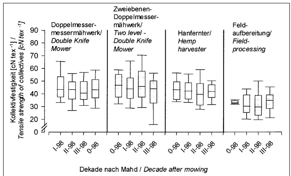
Fig. 3: Tensile strength of fibre bundle collectives during field period after mowing 1998.
