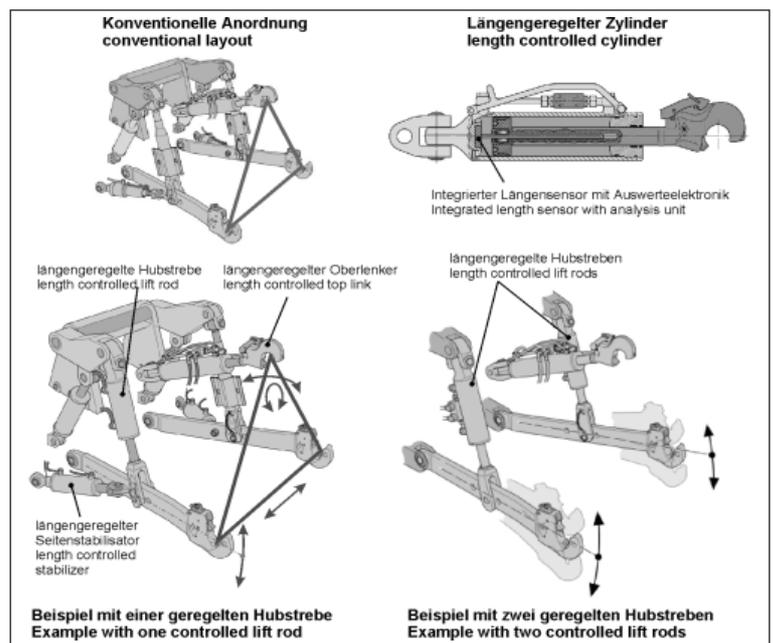
Fig. 1: Different set-ups of the powerlift using hydraulic links
