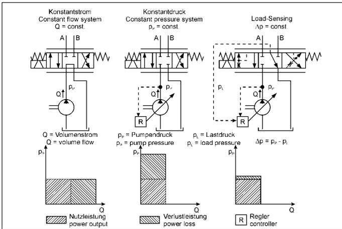
Fig 2: Simplified circuit diagrams and energy balances in part load of conventional hydraulic systems
