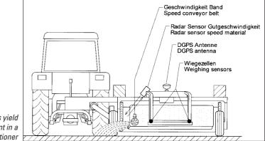
Fig. 1: Continuous yield measurement in a mower conditioner
