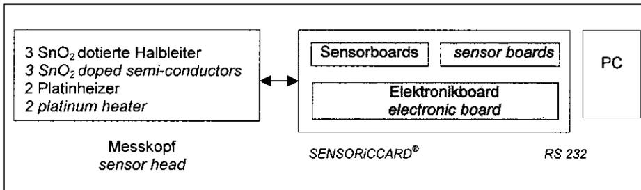
Fig. 2: Schematic view of the Multigas-SENSORiCCARD®.
