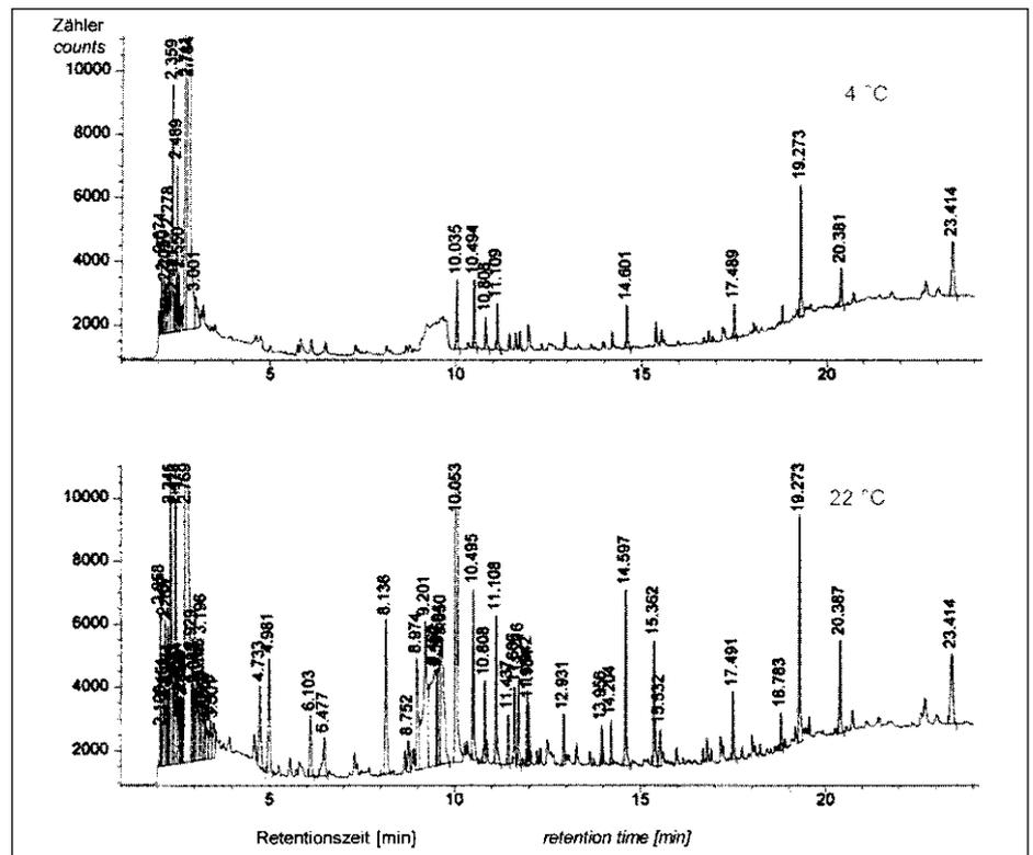
Fig. 4: Headspace analyses of stored apples at 4°C (above) and 22°C (below) recorded by gas-chromatography
