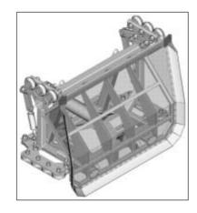
Fig. 2: Moveable push-blade
