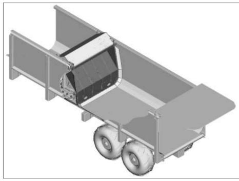
Fig. 1: Transport wagon with moveable push-blade
