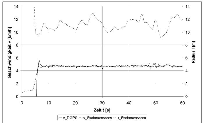
Fig 3: Velocity and radius of a circular path
