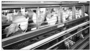
Fig. 1: Completely furnished Eurovent 625+a EU for small-group management for 60 layers
