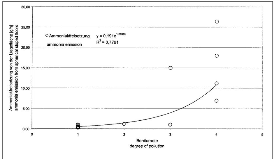
Fig. 2: Ammonia emission from spherically sloped floor and difference degrees of dirtying
