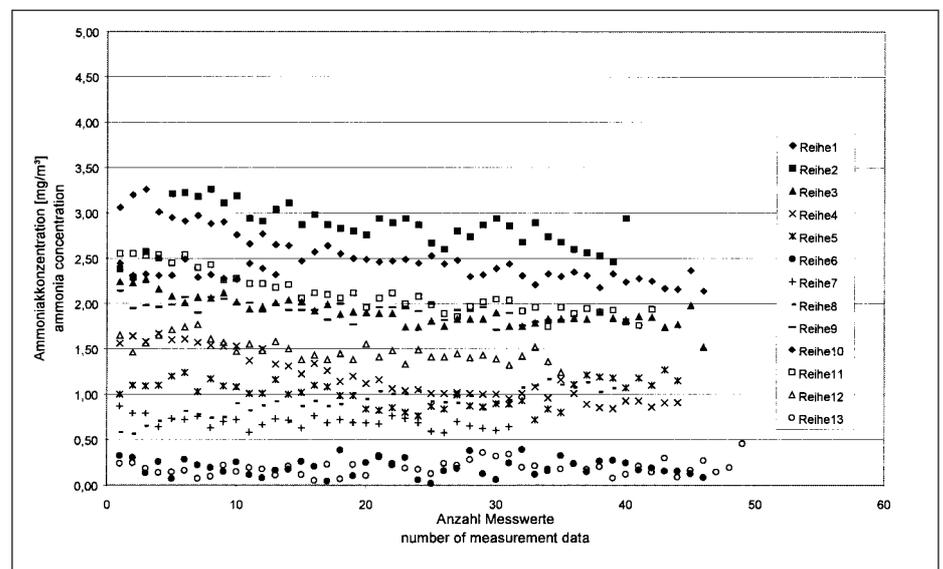
Fig. 1:  $\text{NH}_3$ -concentration over spherically sloped floors in VS I, measured by wind tunnel method.
