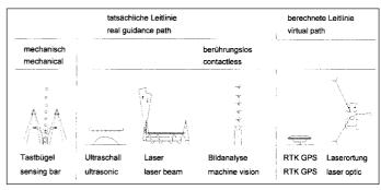
Fig. 4: Automatic guidance systems for farm machines
