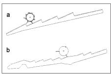
Fig. 2: Rotary elements for grain separation improvement a) Multifinger-Separator-System (Claas) b) Power Separator (John Deere)
