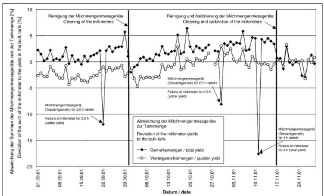
Fig. 2: Development of relative deviation of the milk meters results to milk in the bulk tank
