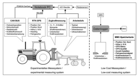
Fig. 1.: Simultaneously used measurement systems for draught force mapping
