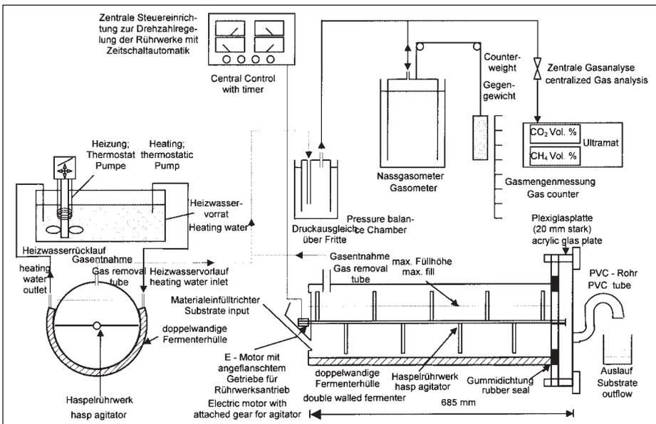
Fig. 1: Scheme of a horizontal Hohenheim laboratory biogas unit (16 l net volume, semicontinuous flow) with hasp agitator, gas storage and gas analysis
