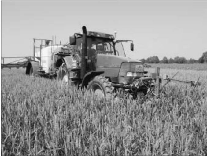
Fig. 2: Sensor in combination with a field sprayer for fungicide application
