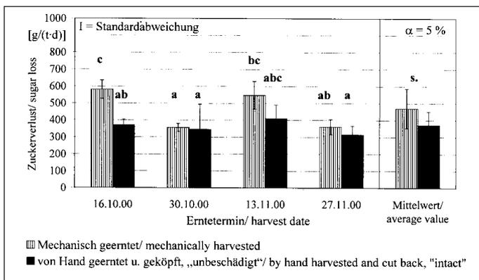
Fig. 3: Calculated sugar loss depending on harvest variant and harvest date in the laboratory tests, duration of storage four days
