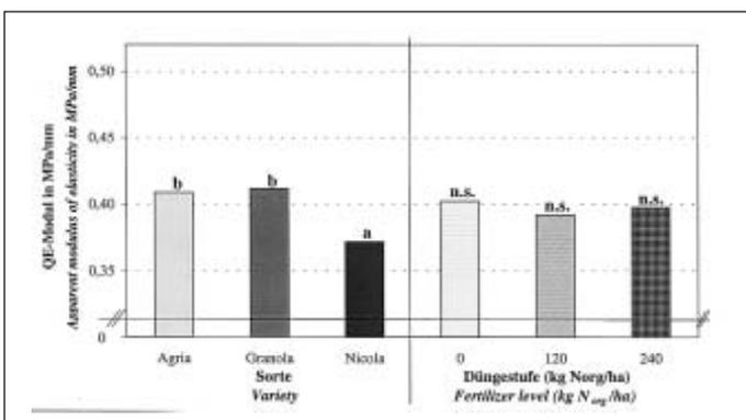
Fig. 3: Apparent modulus of elasticity versus variety and fertilising level - storage time 120 days (penetrometer test 1999)
