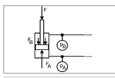
Pressure measurement on both sides of the valve
