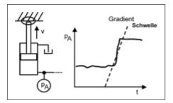
Saltatory pressure change Signal generation Determination of working pressure gradient Evaluation Exceeding a predefined gradient threshold Practical use Recognition of end points, Characteristic intermediate positions and sharply rising pressure Security tests by plausibility checks
