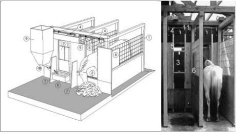
Fig. 1: Design of the feeding station (1 station partition, 2 access gate down/open, 3 access gate up/ closed, 4 cable winch for access gate, 5 guide bar for access gate, 6 antenna, 7 feeding place partition, 8 feed trough, 9 concentrate feed container, 10 concentrate feed dispenser, 11 photo sensor)
