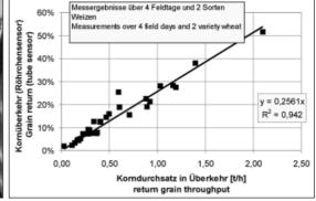
Fig. 3: Measurement results for validation kernel return
