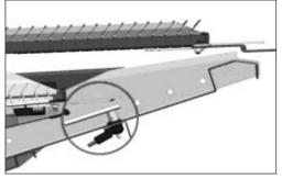
Fig. 1: Tube sensor for detection of the kernel return
