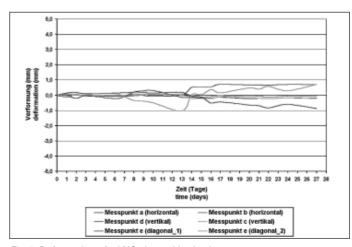
Fig. 5: Deformation of a LNS plate with triarrhena core
