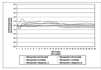
Fig. 4: Deformation of a LNS plate with cardboard-comb core
