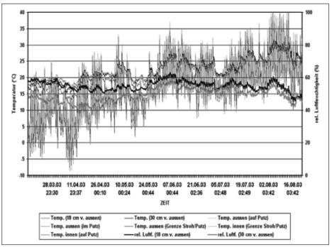
Fig. 1: Course of temperature and moisture in a straw bale wall in Junkershausen (Rhön)
