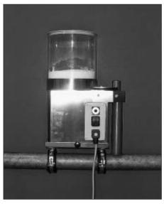
Fig. 3: With the MS Dry Dos by Schippers medicine in powder form can be added easily and very exactly to the dry feed
