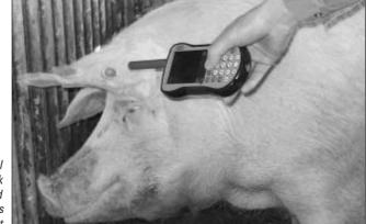
Fig. 1: The hand terminal MilanMPX by Mannebeck has a barcode scanner and full Palm functionality and is housed air and water-tight
