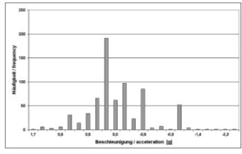
Fig. 4: Histogram of the acceleration values of the Field Scout measurements
