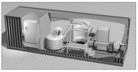
Fig. 2: All components required for decentralized biodiesel production are housed in a transcontainer.
