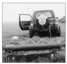
Fig. 2: Measuring instrument EM38 and transport vehicle for the measurement of soil heterogeneity
