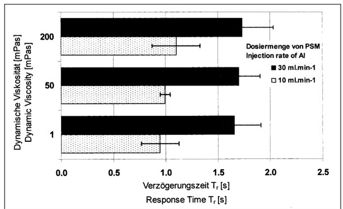
Fig. 3: Comparing lag and response time for three dynamic viscosities of plant protection agent at a constant carrier flow rate (1.97 l min<sup>-1</sup>) and with two flow rates of active ingredient
