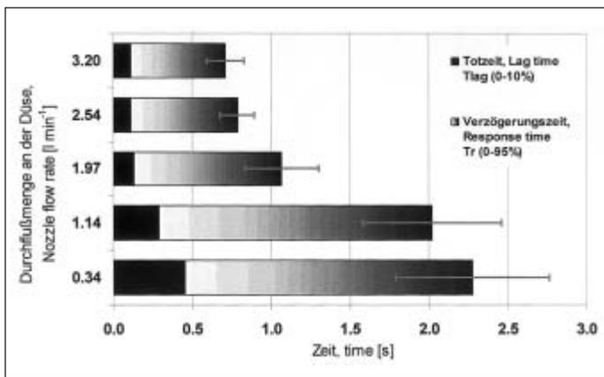
Fig. 2: Comparing lag and response time for different carrier nozzle flow rates at a constant active ingredient flow rate (10.0 ml min<sup>-1</sup>)
