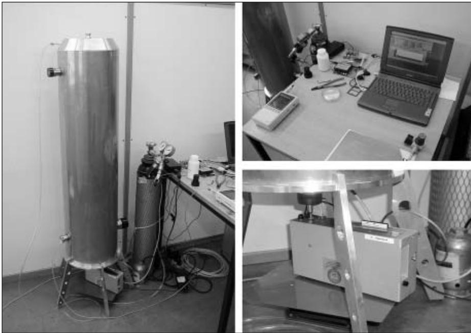
Fig.1: Sedimentation cylinder (left), data acquisition (upper right) and aerosol spectrometer (lower right)
