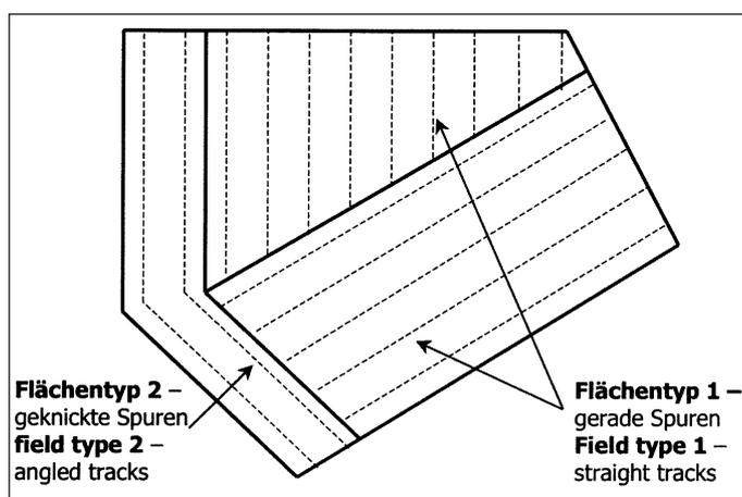
Fig. 1: Part-field with driving tracks and lands
