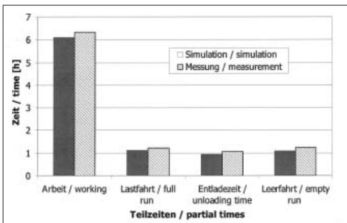
Fig. 3: Comparing measured and simulated results for various partial times
