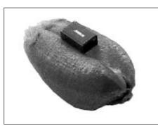
Fig. 2: Size of a RFID-Transponder (mic3®TAG, microsensys, Erfurt) compared to a wheat grain
