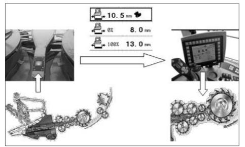
Fig. 3: System integration of the AutoScan sensor
