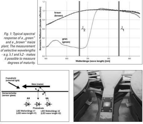
Fig. 2: Principle of measurement for determining the degree of maturity for maize (left) and integration of the sensor system into the maize header of the BiG X forage harvester (right)
