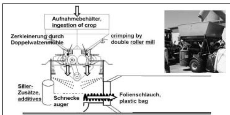
Fig.1: Drawing of an ensiling unit with integrated crimper bagger
