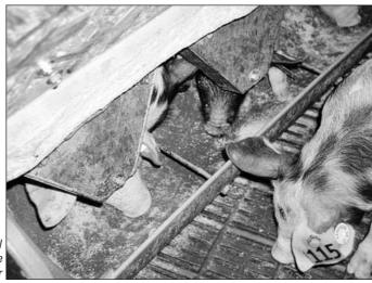
Fig. 2: Detail: bidirectional double-walled feed chute at Tipp-Feeder
