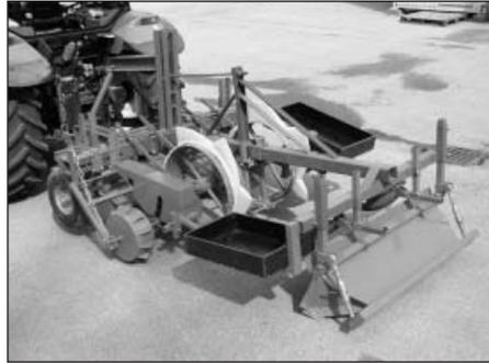
Fig. 2: Vegetable planter modified for horse radish – development stages
